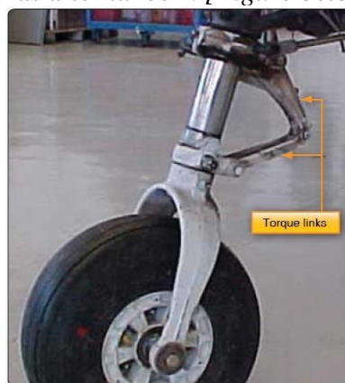
Torque links align the landing gear and retain the piston in the upper cylinder when the strut is extended.
