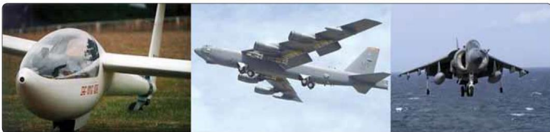
Tandem landing gear along the longitudinal axis of the aircraft permits the use of flexible wings on sailplanes (left) and selects military aircraft like the B-52 (center). The VTOL Harrier (right) has tandem gear with outrigger-type gear.
