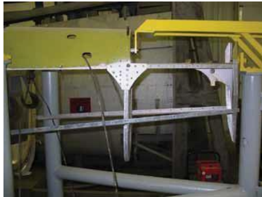
Gussets are used to increase strength.
