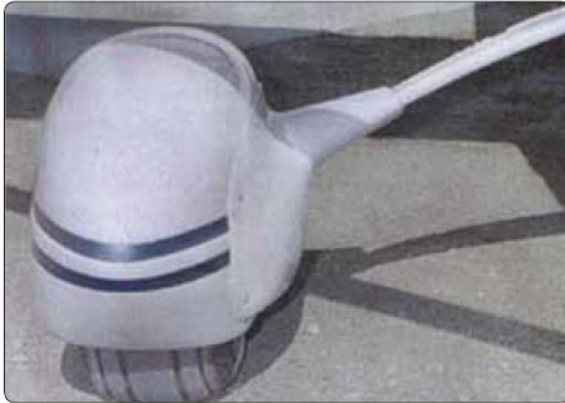
Wheel fairings, or pants, and low profile struts reduce parasite drag on fixed gear aircraft.
