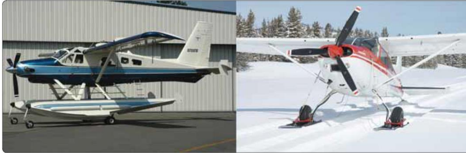
An amphibious aircraft with retractable wheels (left) and an aircraft with retractable skis (right).
