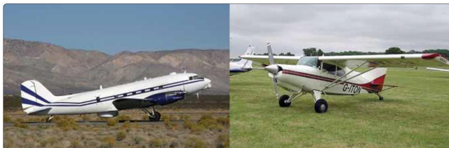
Tail wheel configuration landing gear on a DC-3 (left) and a STOL Maule MX-7-235 Super Rocket.
