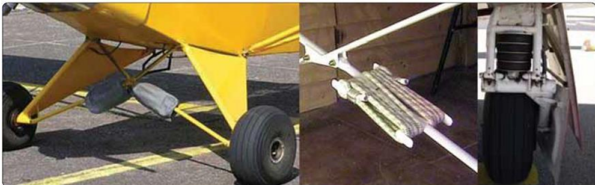
Piper Cub bungee cord landing gear transfer landing loads to the airframe (left and center). Rubber, donut-type shock transfer is used on some Mooney aircraft (right).
