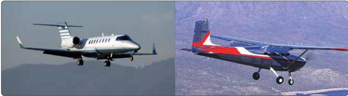
Tricycle-type landing gear with dual main wheels on a Learjet (left) and a Cessna 172, also with tricycle gear (right).
